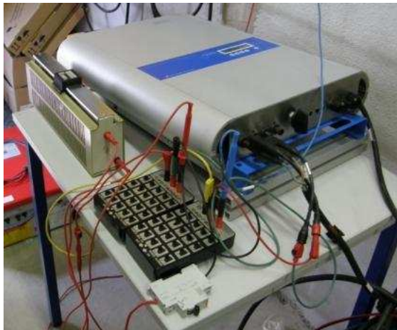
Figure 7: Inverter under test with capacitance between the positive and negative poles and the ground to increase the leakage current
